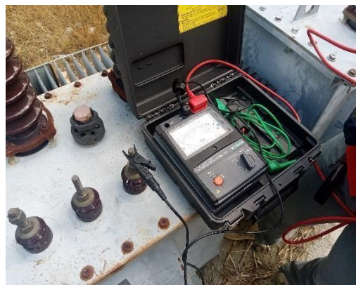
Gambar 2.3 Alat Ukur Insulation Tester (Sumber: PT. PLN PERSERO ULP Selatpanjang)
