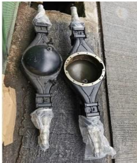
Gambar 4.3: Axle Shart Housing (Sumber: https://www.scribd.com )
