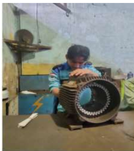
Gambar 2. 53 memasang litroid (sumber: PTPN IV Regional III)
