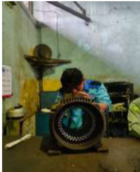
Gambar 2.20 memasang litroid (sumber: PTPN IV Regional III)
