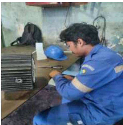
Gambar 2.17 memasang litroid kedalam slot rotor (sumber: PTPN IV Regional III)
