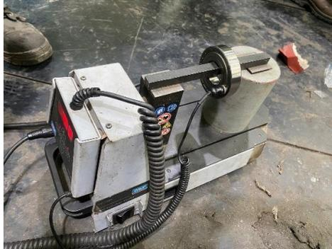
*Gambar 4 12 Heater Bearing*
