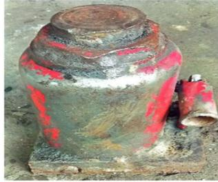
Gambar 4. 9 *Silinder* Hidrolis
