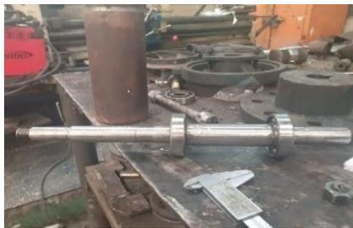
Gambar 4. 11 *shaft* pompa
