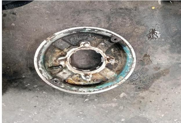
Gambar 4. 17 *Stuffing box pompa sentridugal*
