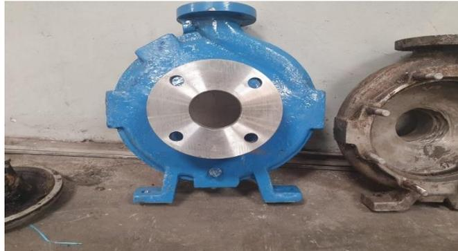
Gambar 4. 15 *Casing* Pompa *Sentrifugal*
