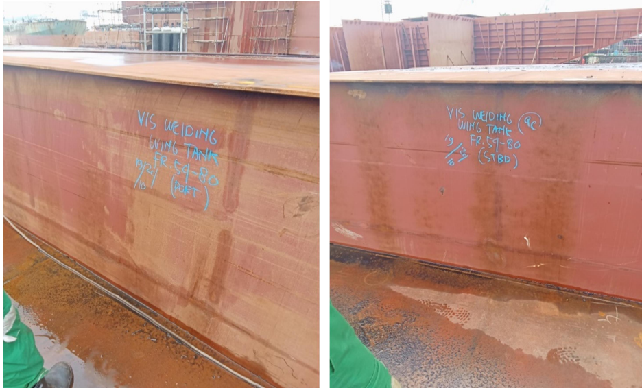
Gambar 2.70 Visual W.I Wing tank
