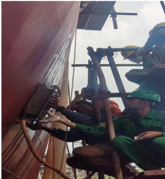
Gambar 2.90 Vacum Test Insert Plate
