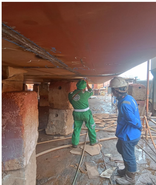
Gambar 2.105 Visual welding bilge
