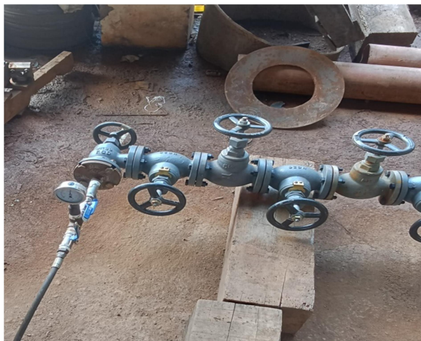
Gambar 2.103 Hydro Test Valve 5k40
