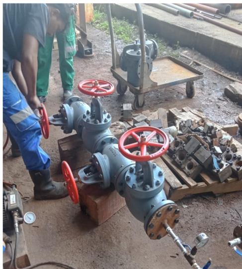
Gambar 2.107 Hydro Test Valve 10K 100
