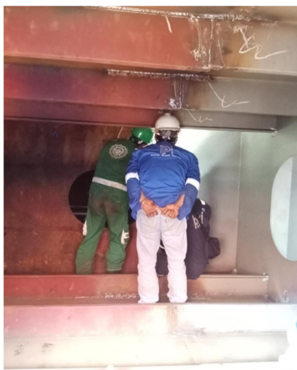
Gambar 2.57 Visual Welding Joint Erection
