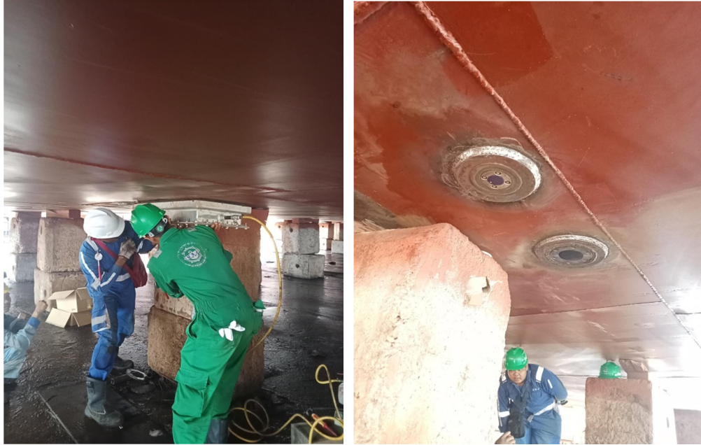
Gambar 2.48 Vacum Test Echosounder
