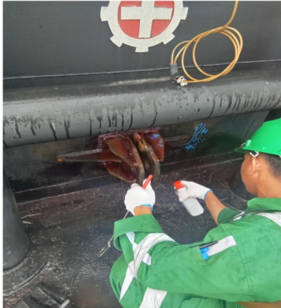
Gambar 2.98 Penetrant Test Bracket
