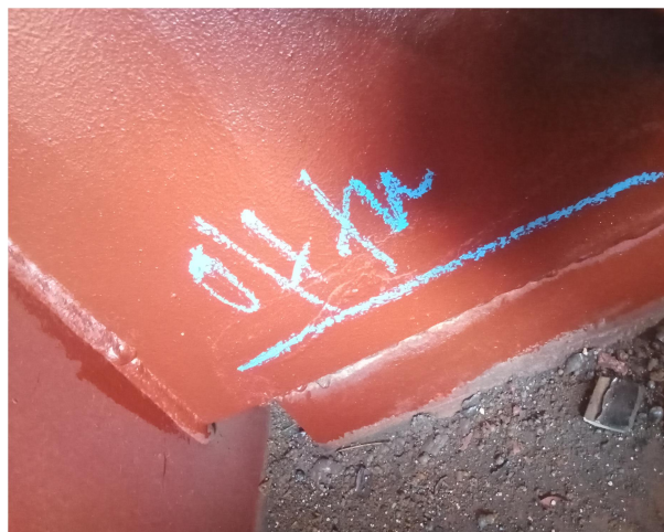
Gambar 2.3 Visual Welding Inspection Cargo
