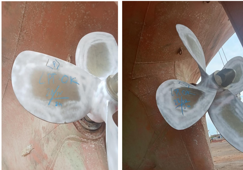
Gambar 2.78 Penetrant test propeler
