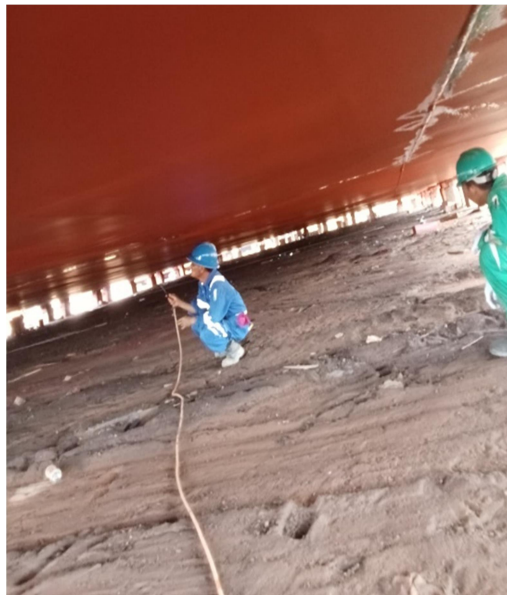
Gambar 2.37 Air Test Void tank
