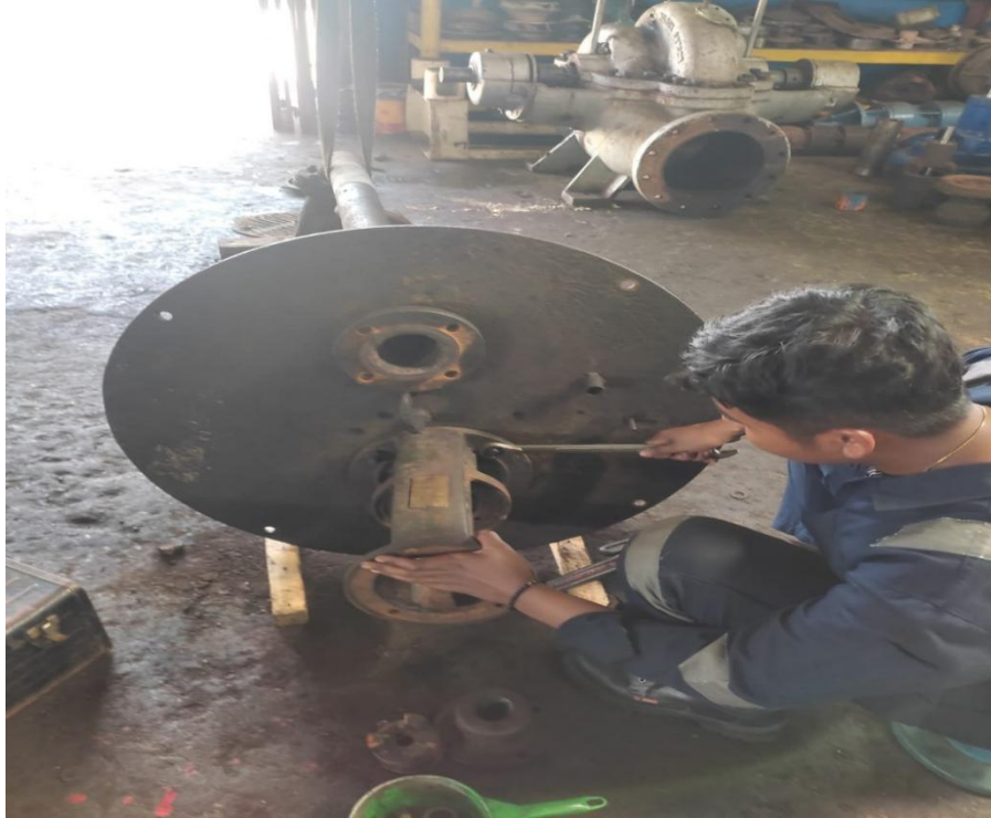
Gambar lampiran 1: maintenance vertikal sump pump
