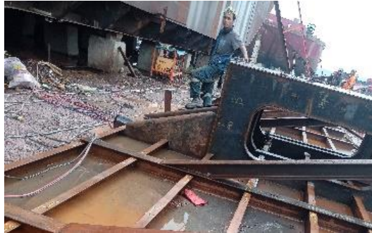
Gambar 2. 17 Visual welding inspection sideboard
