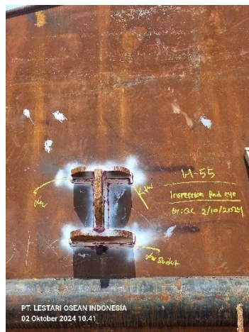
Gambar 2. 47 DYE penetrant test kupingan lifting turning
