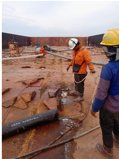
Gambar 2. 61 External air test hull 24
