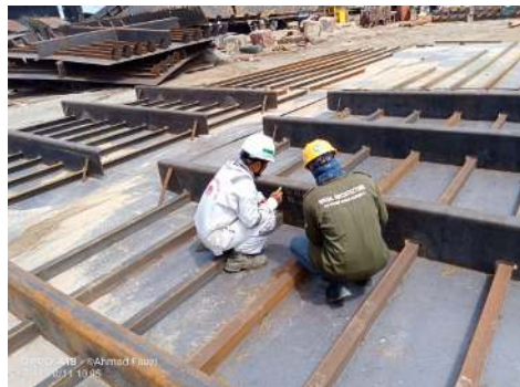
Gambar 2.65 Welding Inpection Long Bhd S/P Tongkang Pelawan Bay 2322
