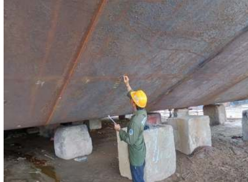
Gambar 2.24 Actual Welding Seam Joint Bottom Shell PSI 2401
