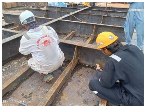
Gambar 2.70 Welding Inspection Longitudinal Bulkhead Tongkang Tomini Bay 2338
