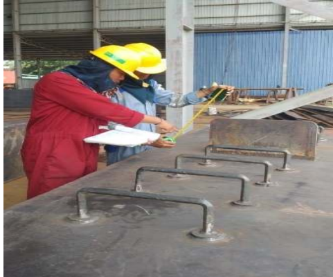
Gambar 2.34 Inspeksi dan Pengukuran Funnel Tug Boat Brighton Dolphin
