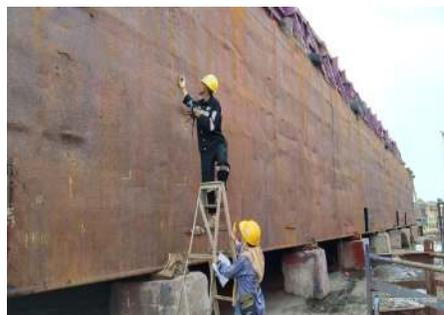
Gambar 2.81 Ultrasonic test side shell
