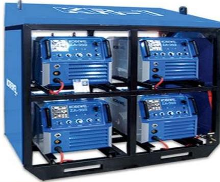
Gambar 3.3.2. SMAW (Shielded Metal Arc Welding)
