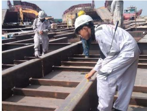
Gambar 3.5.11. Inspection welding
