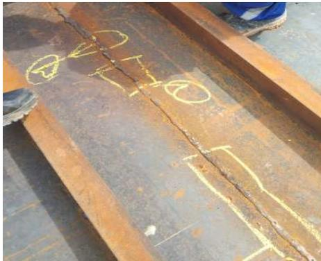
Gambar 2.27 Visual Test Main Deck
