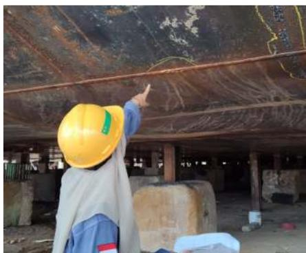
Gambar 2.49 Pengecekan seam joint tongkang
