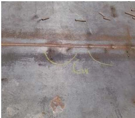
Gambar 2.17 Visual test side shell
