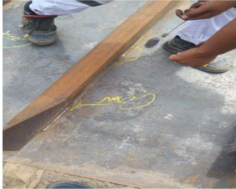
Gambar 2.22 Visual Test dijetty 4 main deck
