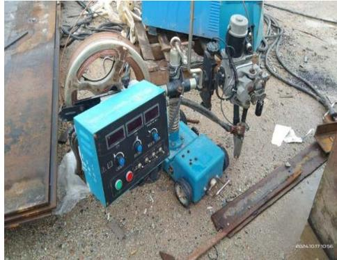
Gambar 3.3.1. Submerged Arc Welding (SAW)
