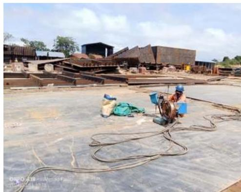
Gambar 3.5.4. Welding Seam Join bottom tongkang
