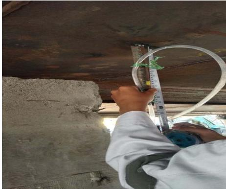
Gambar 2.24 Leveling Test H-162
