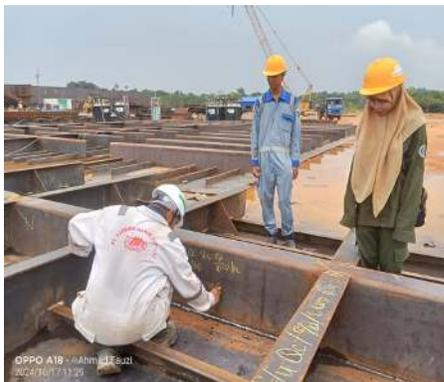
Gambar 2.71 Visual test tongkang main deck h183 Tomini bay 2388
