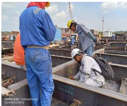
Gambar 2.53 Visual inspection fit up tongkang H-183
