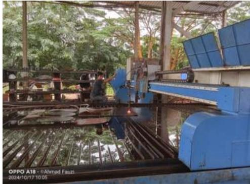
Gambar 3.4.7. CNC (*Computer Numerical Control*) Plasma
