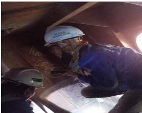
Gambar 2.13 Visual Test Tangki freshwater Tug Boat
