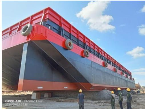
Gambar 2.11 Proses Launching Tongkang PSI 2401
