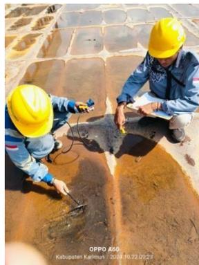
Gambar 2.28 Ultrasonic Thicknes (UT)
