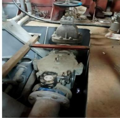
Gambar 2.53 Pengecekan Kebocoran pipa Sea Chest
