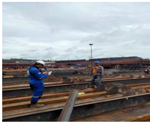
Gambar 2. 4. Fit Up Long & Trans Bulkhead
