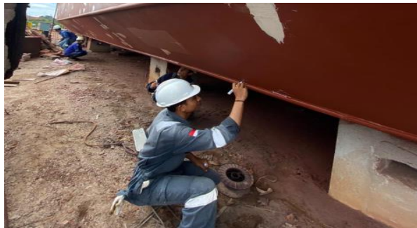
Gambar 2. 168.Final Weld Inspection
