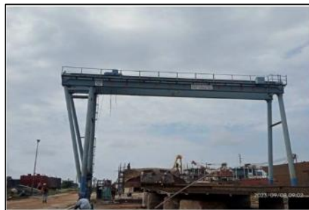
Gambar : 1.5 Gantry Crane
