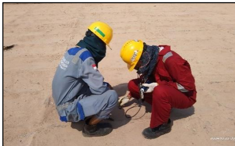
Gambar 2.77 : Proses UT main deck
