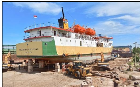
Gambar 2.49 : Proses docking metode slipway
