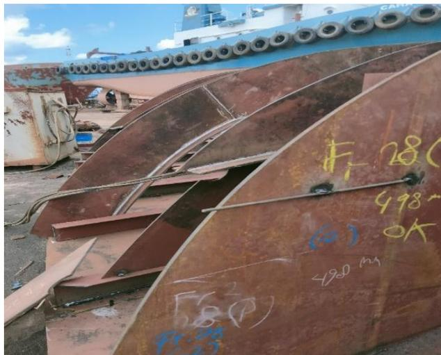
Gambar 2.35 Visual welding inspect bilge Tugboat
