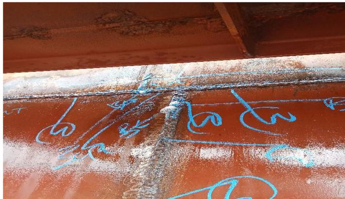
**Gambar 2.11** *Visual welding inspect side sheel*
