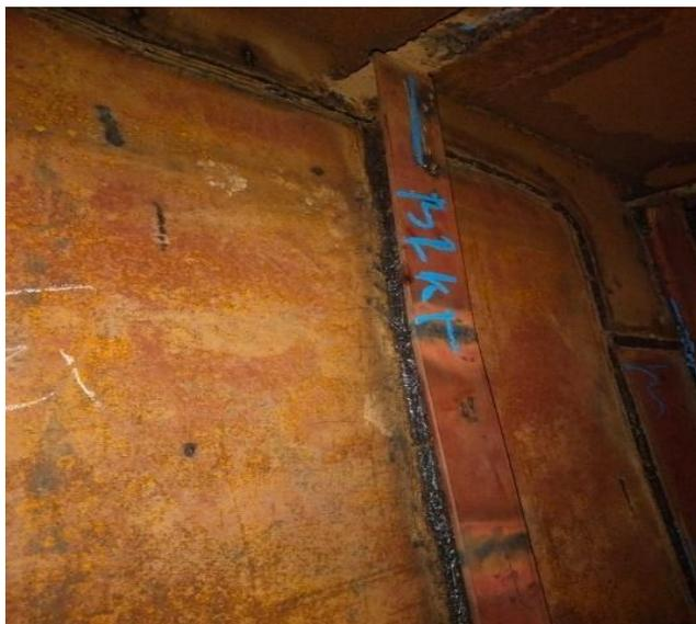
Gambar 2.81 *Visual welding inspect kapal cargo*
