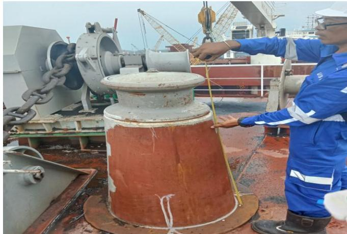
Gambar 2.14 *Visual Welding Inspect roller fairlead*
