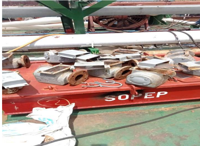
Gambar 2.67 Inspection air vent head
