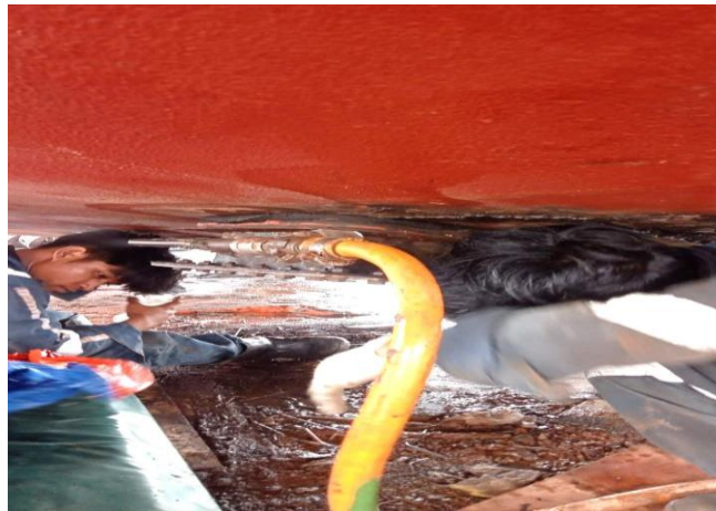
Gambar 2.29 Proses vaccum test
