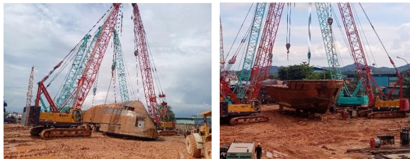
Gambar 2. 46 Lifting turning TB hull 055
