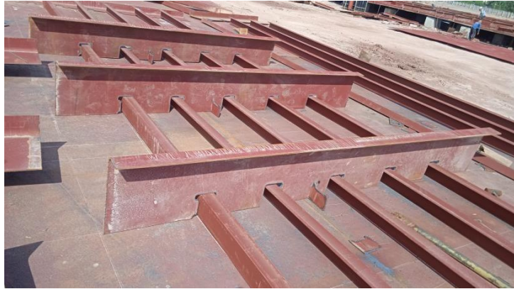
Gambar 2. 30 pengecekan fit-up L.bhd
