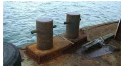
*Gambar 3.17 Double bollard*
