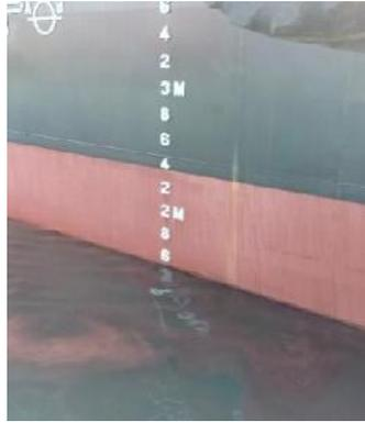
Gambar 3. 14 Kondisi draft kapal saat ballasting
