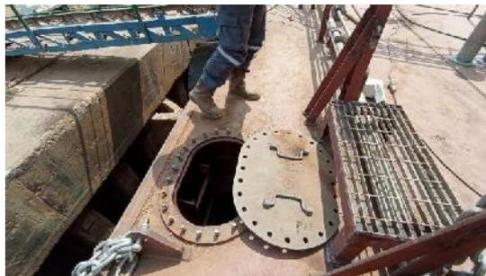
Gambar 2. 47 Ballast tank
