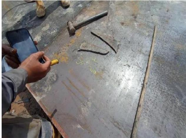
*Gambar 2. 4 Proses tracing plat marine*
