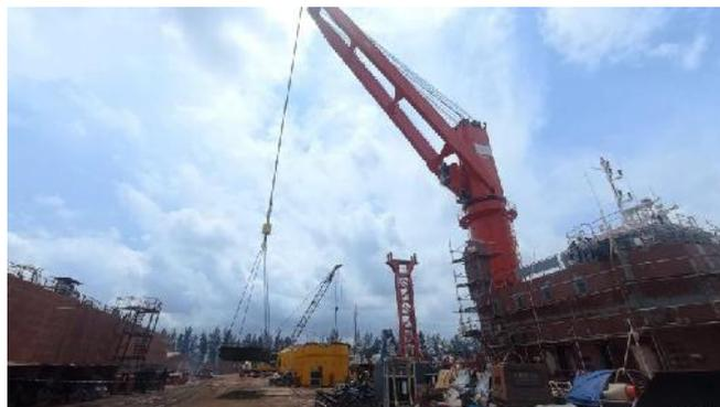
Gambar 3. 15 Proses load test crane
