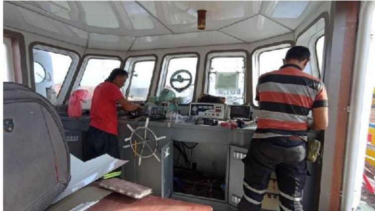
Gambar 2. 38 Pemasangan electrical equipment di wheelhouse tugboat
