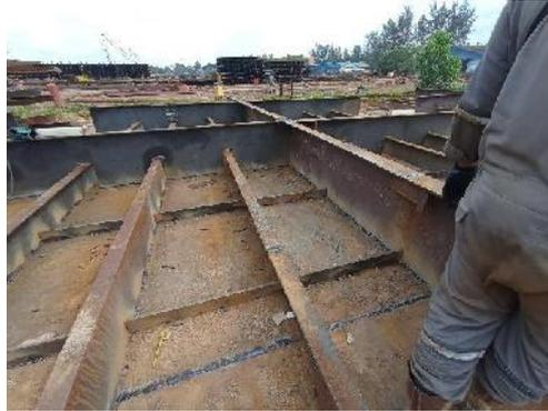
*Gambar 2. 23 Panel main deck crane barge*
