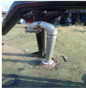
Gambar 2. 98 Gooseneck air vent tugboat MBP 3232
