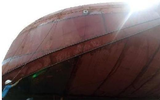
*Gambar 2. 28 Proses eksternal Air Test cargo barge*
