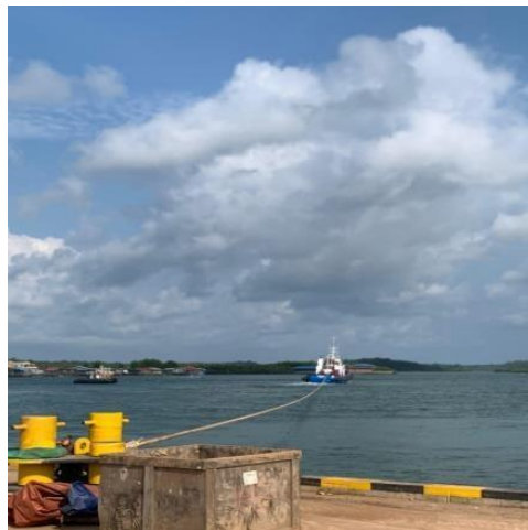
Gambar 2. 48 proses bollard test
