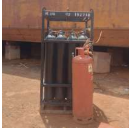
Gambar 1. 18 Oxygen dan LPG (Liquefied Petroleum Gas)
