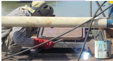
Gambar 2.20 Pengelasan top stering room
