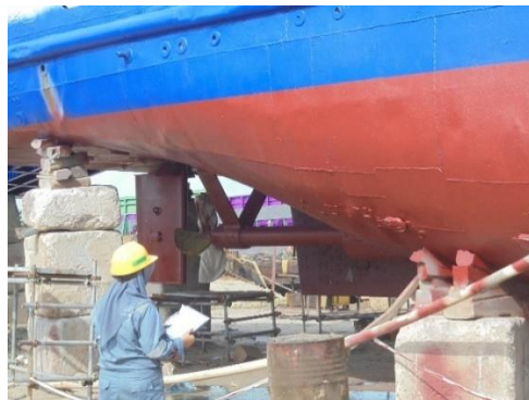
Gambar 2.39 Inspek install zinc anode new
