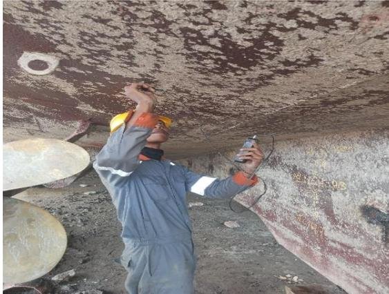
**Gambar 2.21** *Ultrasonic Test bagian Buritan*
