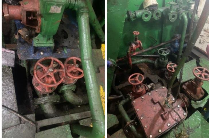
Gambar 3.1. *Pipa Induk (Main Pipeline)*
