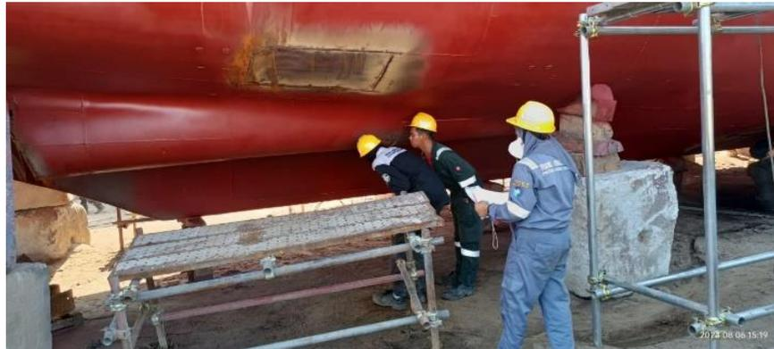
*Gambar 2.20 Pemasangan Pipa Air Tawar Dan Drawing Replating Bottom*
