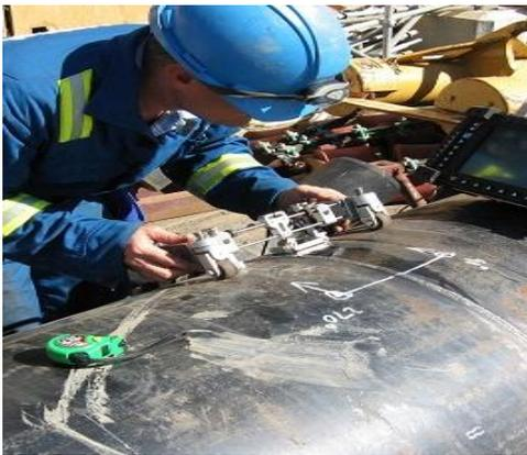
Gambar 2.6 test ultrasonic
