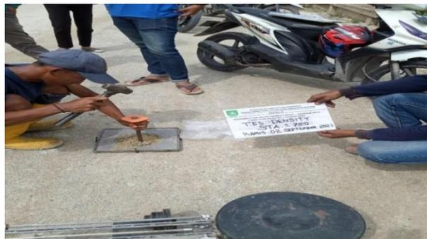
Gambar 3.18. Pengujian Sand Cone Base A
