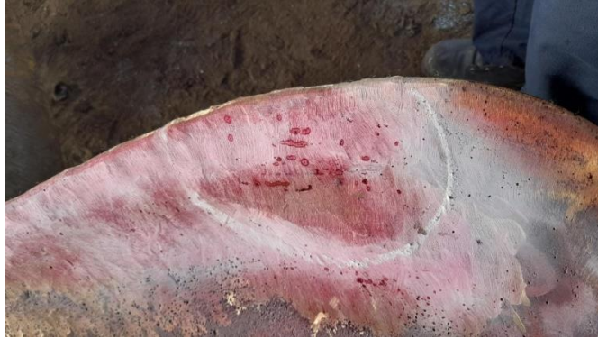
Gambar 2.20 Colour Check Daun Propeller KM Kirana III
