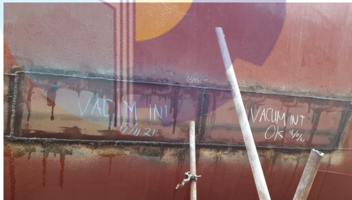
Gambar 2.10 Area Replating Lajur Bilga Bagian Portside Frame No. 60-65 Kapal Trifosa pasca Vacum Test
