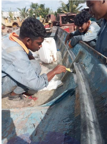
Gambar 2.59 Proses Laminasi Gading Speed Boat
