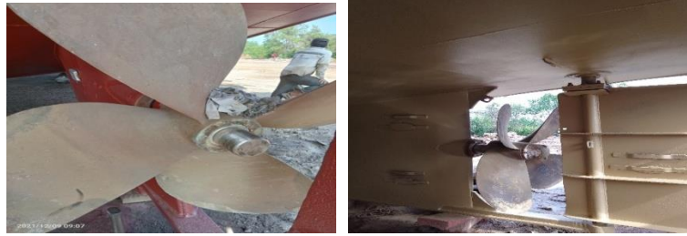
Gambar 3.9 Fixed Pitch Propeller (FPP)
