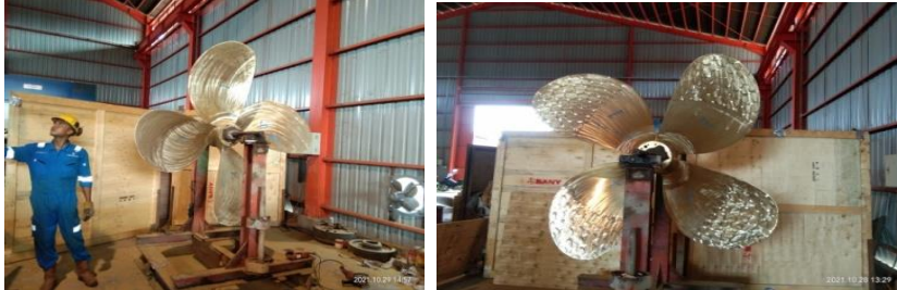
Gambar 3.7 Proses Balancing Propeller
