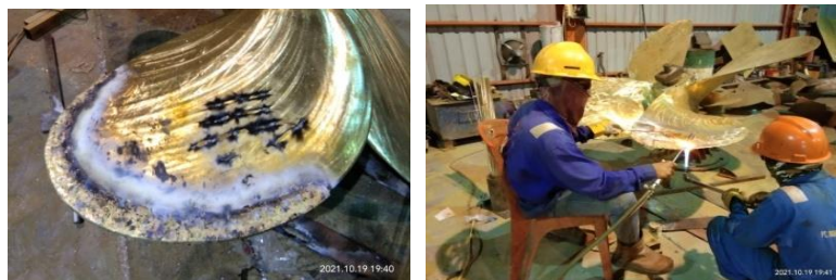
Gambar 3.5 Proses Build- up Propeller
