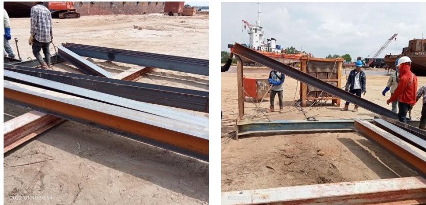
Gambar 2.46 Proses perakitan Sideboard BG. Taurus
