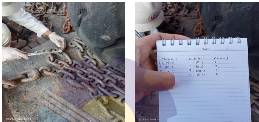
Gambar 2.39 proses kalibrasi rantai jangkar TB. Satia Mulia 11
