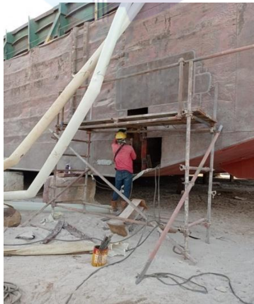
Gambar 2. 59 Insert Plate Sideshell
