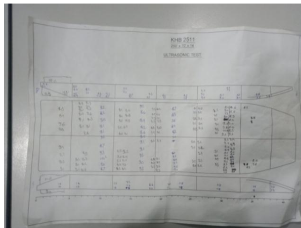
Gambar 2. 56 General ARRANGEMENT Ultrasonic Test (UT)
