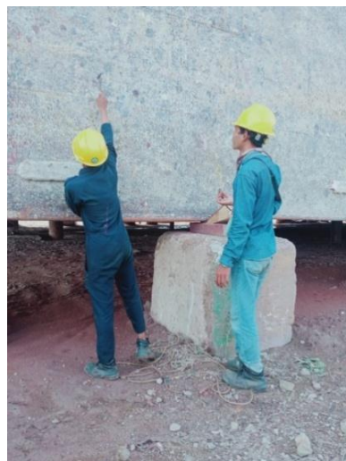
Gambar 2. 62 Ultrasonic Test bagian Sideshell
