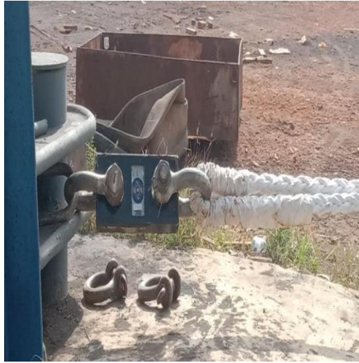
Gambar 2. 43 Proses bollard pull test
