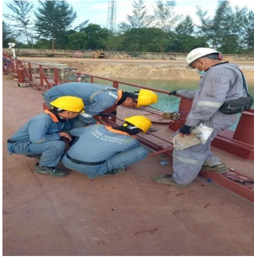
Gambar 2. 11 Sounding bagian startboat
