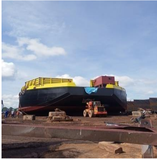
Gambar 2. 4 Launching kapal tongkang jingxi 02
