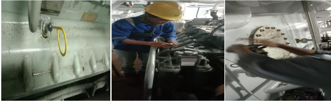
Gambar 2. 33 Proses persiapan startup main engine
