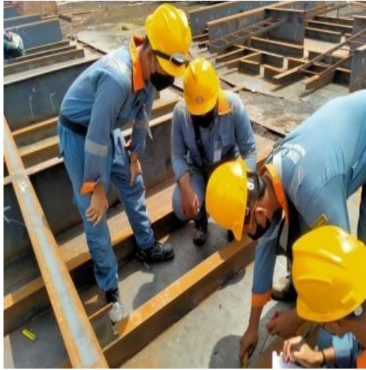
Gambar 2. 3 Proses inspect welding transverse bulkhead
