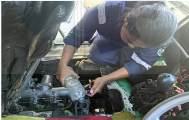
Gambar 4.12 Penambahan Air Radiator
