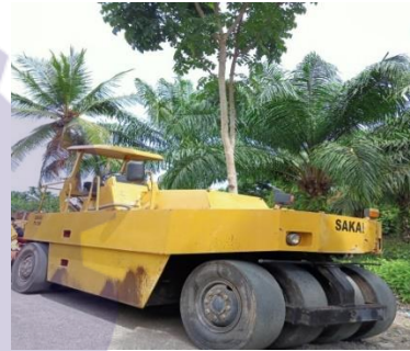
Gambar 2.9 Pneumatic Tired Roller
