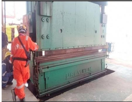
Gambar 2. 6 Mesin Bending.
