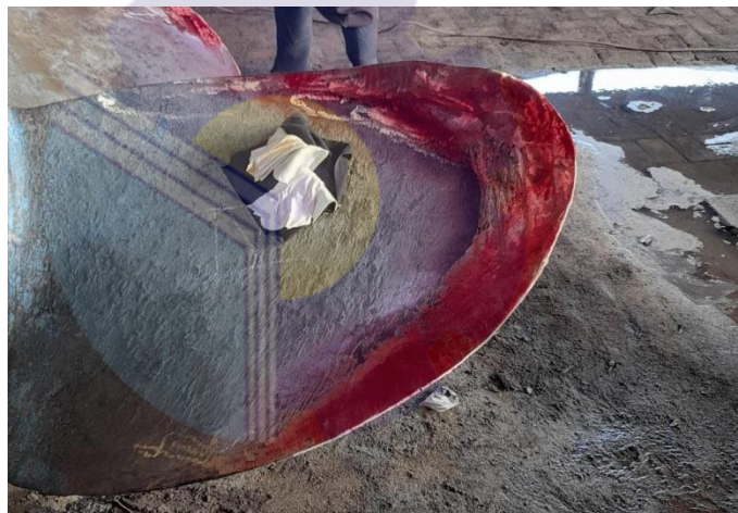
Gambar 2.21 Penetrant Test Daun Propeller
