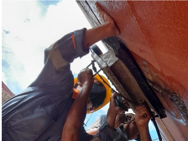
Gambar 2.9 Proses Vacum Test
