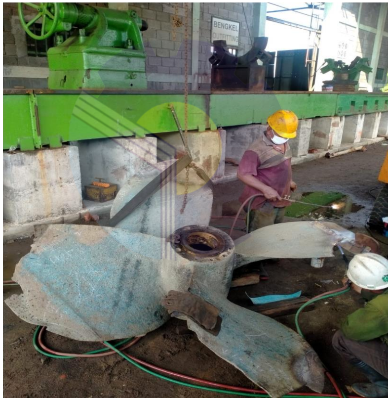
Gambar 3.11. Proses beri tanda marking daun propeller
