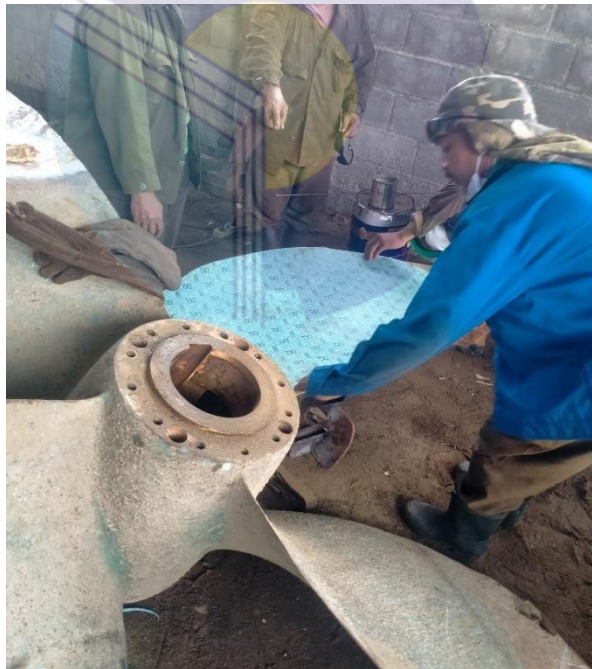
Gambar 3.6. Proses marking/ penandaan daunpropeller
