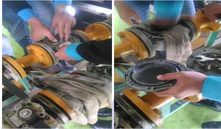
Gambar 2.6 pergantian filter kit
