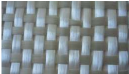
Gambar 2.1 Susunan Serat gelas Woven Roving (Carli, et al, 2012)
