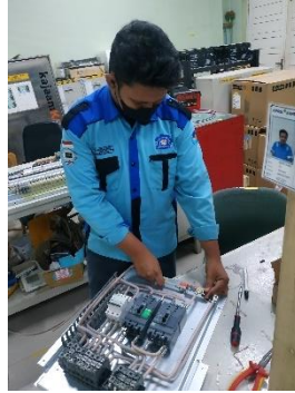
Gambar 2.18 Lanjutan Merangkai Power Distributed Panel
