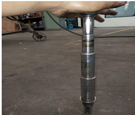
Gambar 4.3 shaft pompa sentrifugal
