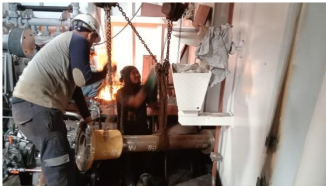
Gambar 3.16 Lifting intermediate shaft to coupling engine and coupling as
