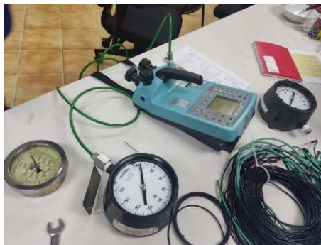
Gambar 2.11 Kalibrasi Pressure Gauge
