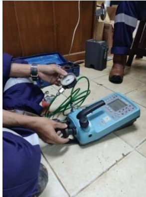
Gambar 2.14 Kalibrasi Pressure Gauge
