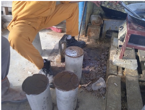
Gambar 3. 9 Caping sampel Beton
