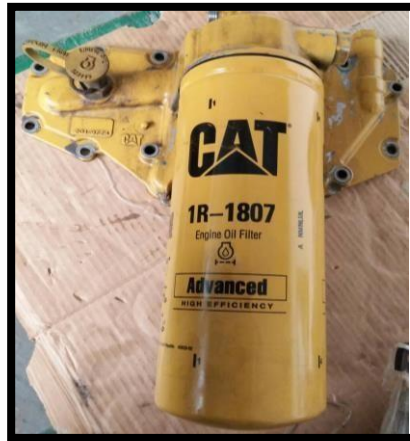
Gambar 4. 5 Oil Filter with Bypass Valve Sumber : PT.Besmino Materi Sewatama
