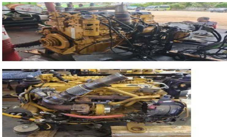
Gambar 4. 11 Engine C7 Caterpillar (sumber PT.Besmino Materi sewatama)
