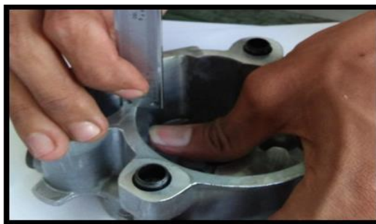
Gambar 4. 19 Pengukuran Depth of the bore for the gear Sumber: PT. Besmindo Materi Sewatama
