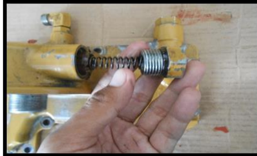
Gambar 4. 26 Plug,plunger dan spring
