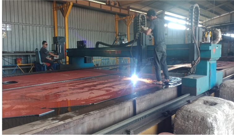
Gambar 2.24 : proses kerja Plasma Cutting
