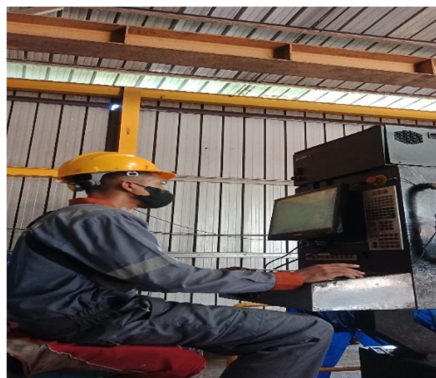
Gambar 2.25 : Teknologi computer plasma cutting
