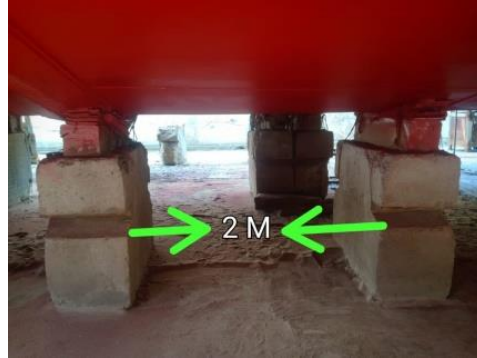
Gambar 3.16 jarak antar keel block
