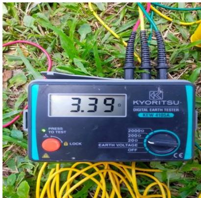
Gambar 3.3 Alat ukur grounding (Earth tester)
